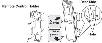
Mounting Screws 5/32 x 5/8" (4 x 16 mm) (included)  To prevent loss of the remote controller, you can connect the remote controller to the holder by passing a string through the remote controller and attachment hole.
